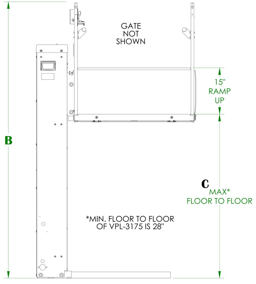
**NOTES: 1) ACCESS RAMP & PLATFORM GATE CAN BE MOUNTED ON EITHER SIDE OF THE PLATFORM**
